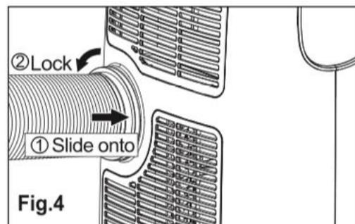
**3. Installation of the hose to a window/balcony without the window mount**
