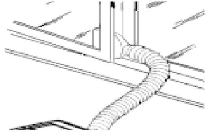
**4. Installation of the hose to a window with the window mount**
