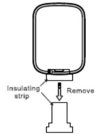
Replacing the battery:
